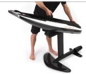
Slip the board on top of the drive unit and fasten the connection by pressing down the black locking handle.
