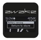
When the Flex BP state of charge is very low, the Flex BP will switch to SLOW mode to save battery charge and ensure that there is enough charge left to make it back to shore
