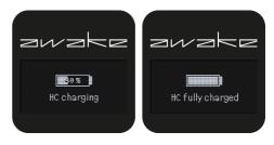
The charge remaining can be found at any time in the top right corner of the display when the Flex HC is powered on.
