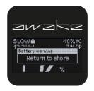
When the Flex BP state of charge is very low, the Flex BP will switch to SLOW mode to save battery charge and ensure that there is enough charge left to make it back to shore.
