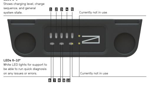
\*The bottom LEDs (6-10+) on the Flex BPs with **LED display v.1** consist of three "LED containers" with two separate lights in each.
