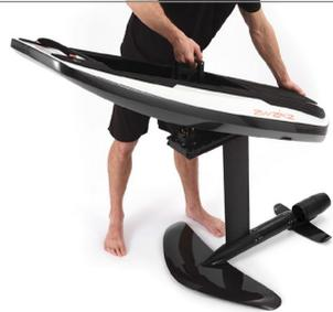
3. Slip the board on top of the drive unit and fasten the connection by pressing down the black locking handle.
